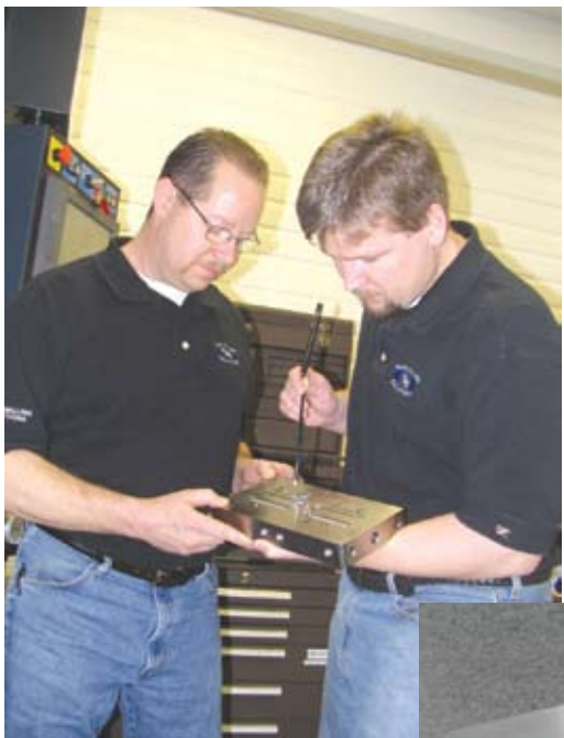
Corey Greenwald (above right) and Kevin Hunter inspect the details of a mold block produced on one of the shop's Makino V56 vertical machining centers. This block (right) is made of hardened H13 tool steel. A 1.0-mm diameter ballnose end mill with a 12:1 length to diameter ratio was the smallest tool used in this project, which substantially reduced EDM and polishing operations for the customer.
