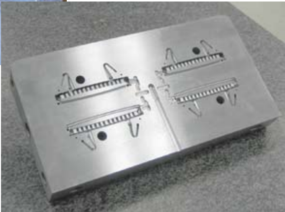
Corey Greenwald (above right) and Kevin Hunter inspect the details of a mold block produced on one of the shop's Makino V56 vertical machining centers. This block (right) is made of hardened H13 tool steel. A 1.0-mm diameter ballnose end mill with a 12:1 length to diameter ratio was the smallest tool used in this project, which substantially reduced EDM and polishing operations for the customer.
